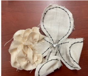
Figure 1. Muslin prototype of SMA wire corded petals.
